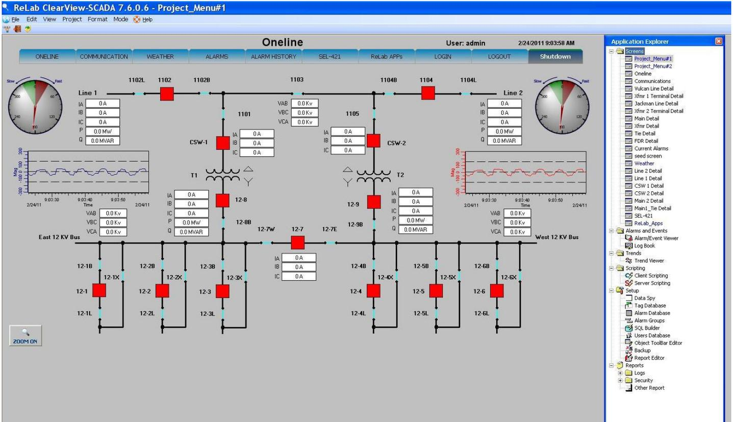
Figure 1 – Example of Substation One-line
